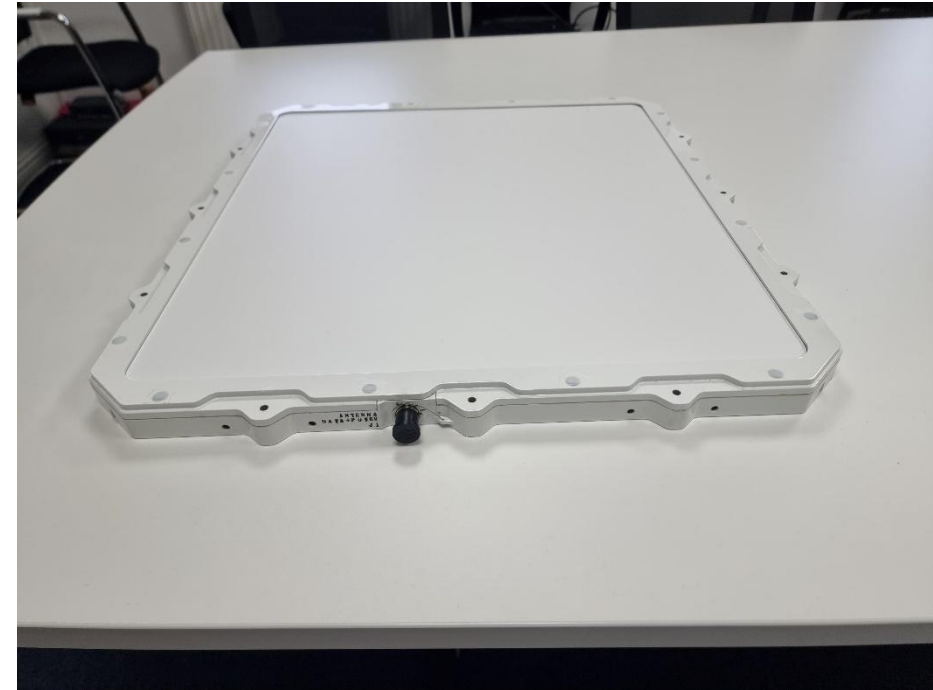
Roof-Integral High-Performance Terminal (IP67 + EN 50155)
